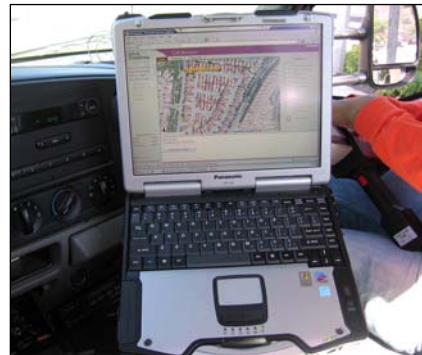
Figure 5: Mobile application provides field personnel access to GIS, assets, work orders, and documents.
