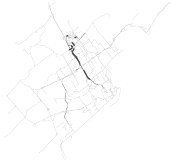
Figure 8: The enlarged displacement space (part of an origin-destination survey) for Charlesbourg, Québec. All linear elements show actual displacements along the road system. The thicker and darker the line, the more frequent the displacements along that segment of road and the more reinforced that element of the space.
