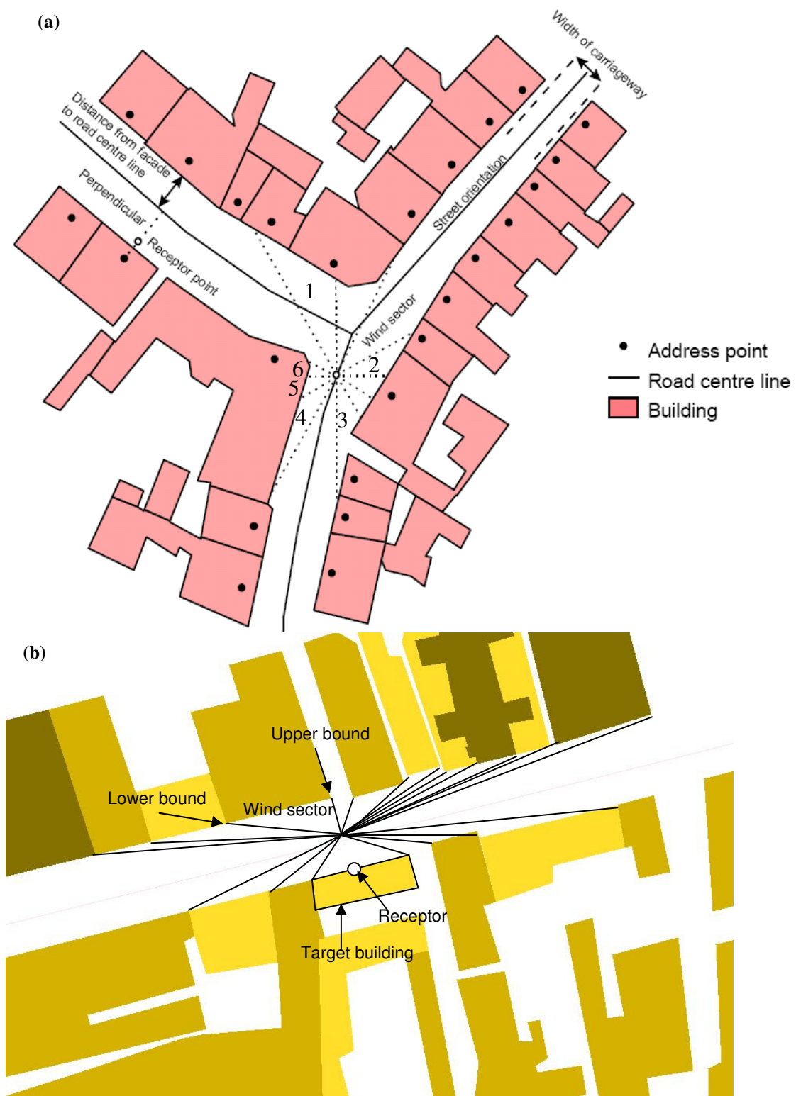
Fig. 2. Wind sectors generated from the urban landscape model by (a) Jensen (1998) and (b) the present study.
