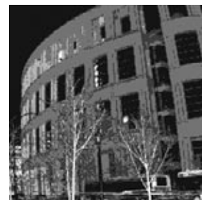
Figure 7.4. Ground-based LIDAR image. Courtesy of Optech
