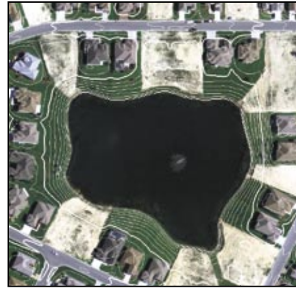
Figure 3.6. LIDAR contours with breaklines and smoothing. Courtesy of Marion County, Florida; Space Imaging; and Jones Edmunds & Associates
