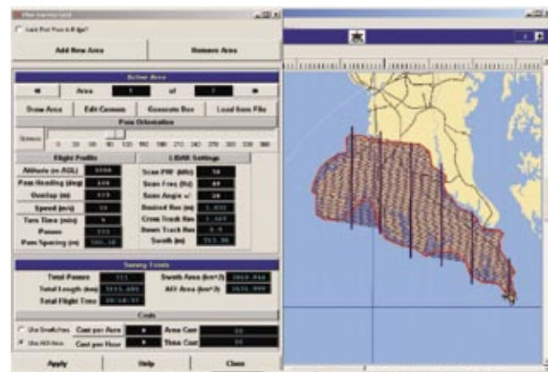
Figure 1.2 Sample LIDAR flight plan.
