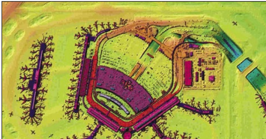
Figure 4.3. Illustration of final bare earth and aboveground classifications at Chicago's O'Hare Airport. Courtesy of the Cook County Office of Technology
