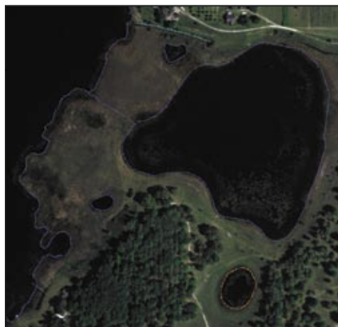
Figure 3.9. The 2-D breaklines in the Marion County, Florida project mosaicked on digital orthophotography created using an ADS40 digital camera. Courtesy of Marion County, Florida; Space Imaging; and Jones Edmunds & Associates
