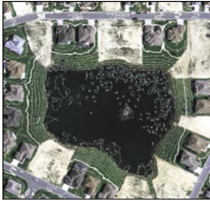
Figure 3.5. LIDAR contours without breaklines and smoothing. Courtesy of Marion County, Florida; Space Imaging; and Jones Edmunds & Associates
