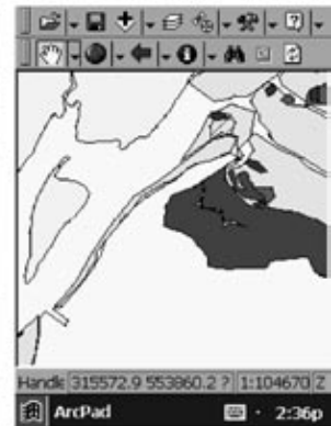
Using ESRI's ArcPad™ on a PDA to connect to an ArcIMS map service and view map data in the field. (Author)
