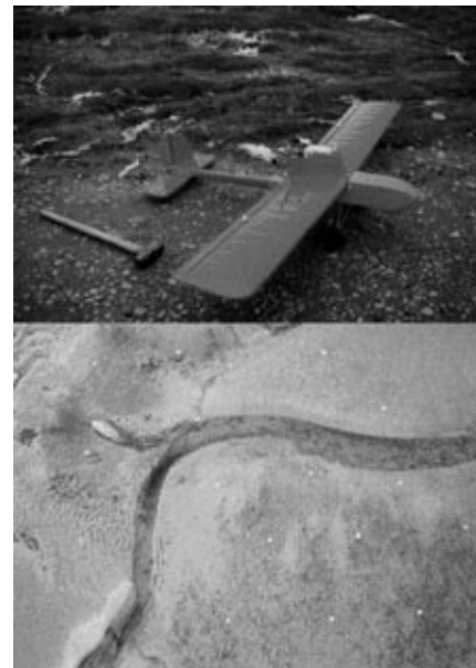
Figure 18 – A Model Airborne Platform and a 35mm Aerial Photographic Print Captured with a 35mm SLR Camera (courtesy of the Author)
