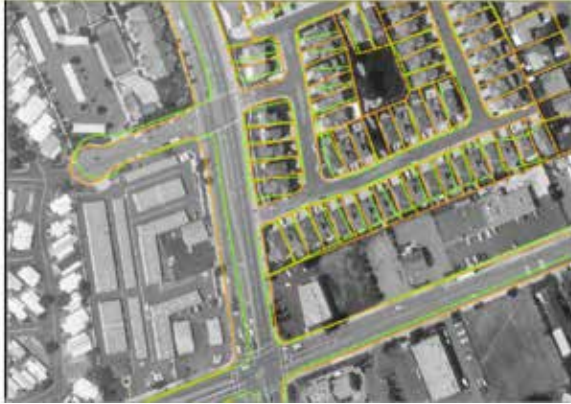
Figure 11. Land parcels can be adjusted to match orthophotography, however, the creation of the orthos should be supervised by a licensed surveyor.
