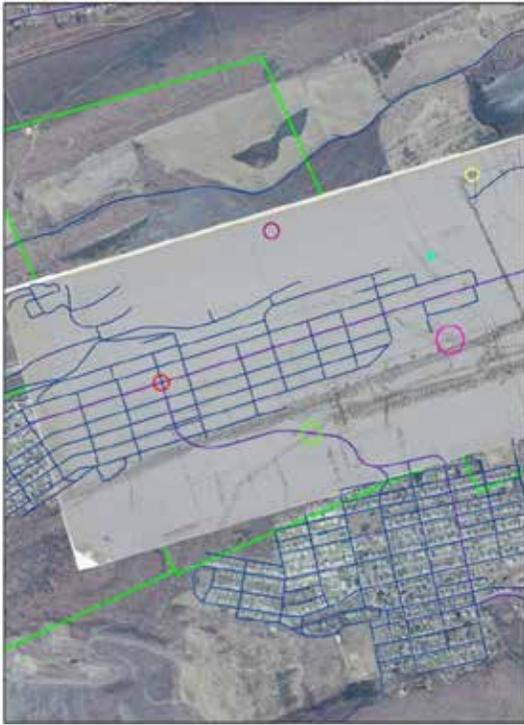
**Figure 2:** shows the location of various georeferencable features on an underground mine map including road intersection (red), bridge (green), building (pink), grid line (purple), mine entrance (yellow), and municipality boundary (blue arrow).
