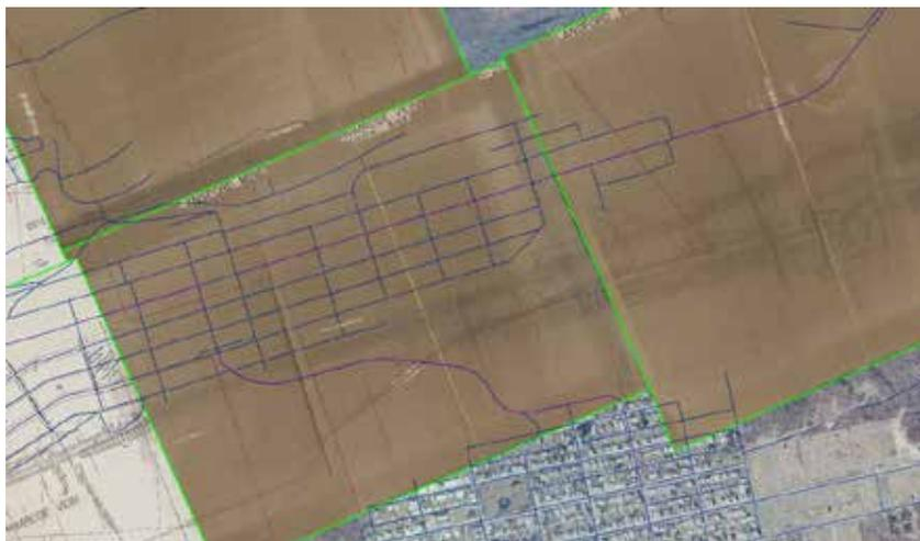
**Figure 4:** shows an example of how underground mine maps are footprinted so that only the desired portions of each map are displayed.
